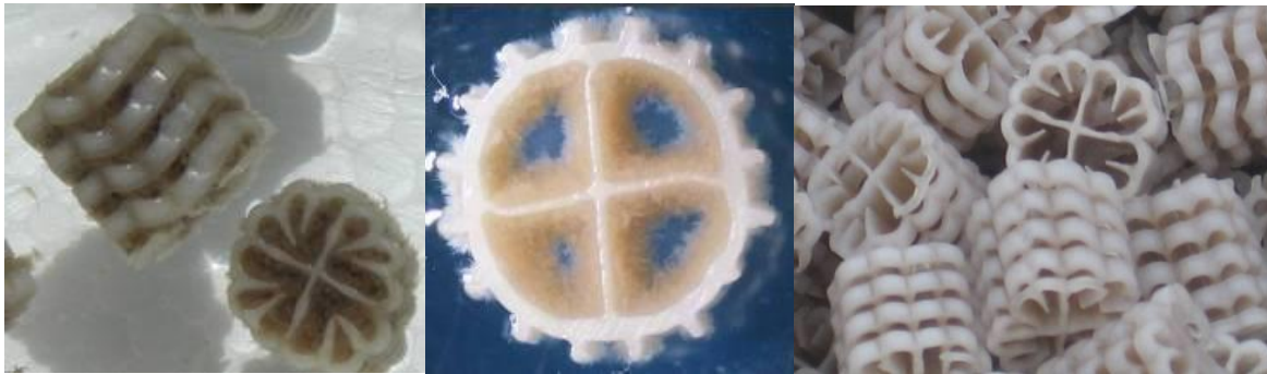
FIGURE -4-10 : BIOMASS CARRIERS IN MBBR PROCESS
